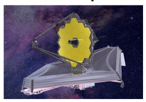
The telescope is the largest and most complicated ever to be launched. It was so large it had to be folded up in its Ariane 5 launch vehicle. Then, in a process lasting 15 days, it unfolded into its final deployed state.
